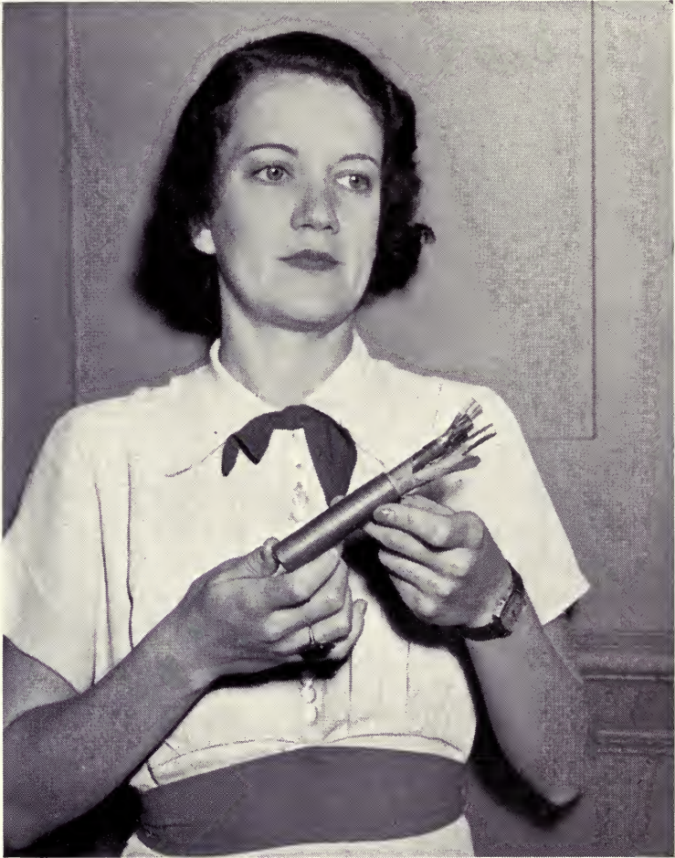
Fig. 44. Piece of Co-axial Cable. The two large tubes can be used for television circuits and the eight other wires are for signaling and control circuits
